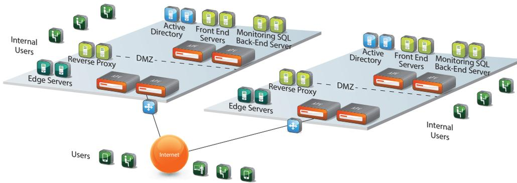
Figure 1: APV Series application delivery controllers in an AD RMS architecture
